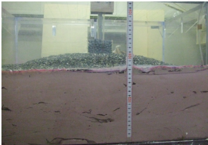
改良後地盤高の様子(重さ2.18kg, 載荷圧1.89kN/m 2 )
